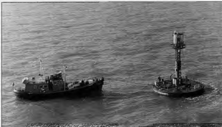
Between 1987 and 1995 the Varne lightvessel was replaced by a large automatic navigation buoy. The Trinity House buoy tender Lodesman is here seen working at the Varne during this period. In the end these buoys proved too uncomfortable and difficult to work on in any kind of sea and they were nearly all withdrawn and scrapped.
