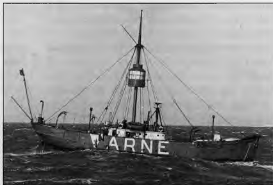
Lightvessel No.65 was typical in design of those stationed at the Varne in earlier years. This picture taken in 1958 shows her acting as relief vessel very shortly before the end of her career. It illustrates also the sea conditions that are only too frequently experienced at the eastern end of the Channel.
