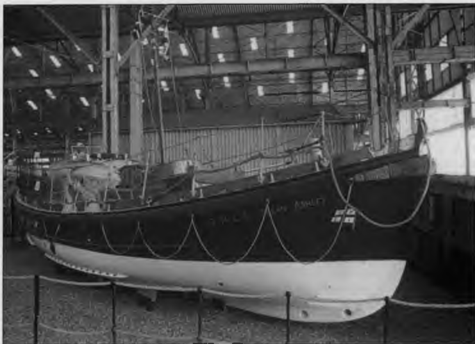
RNLB Susan Ashley - one of a class four 41ft lifeboats built for slipway launching
